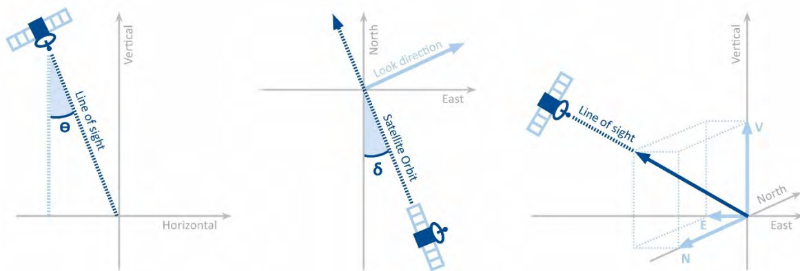
Figure 16: Geometry of the image acquisitions along the ascending orbit.
