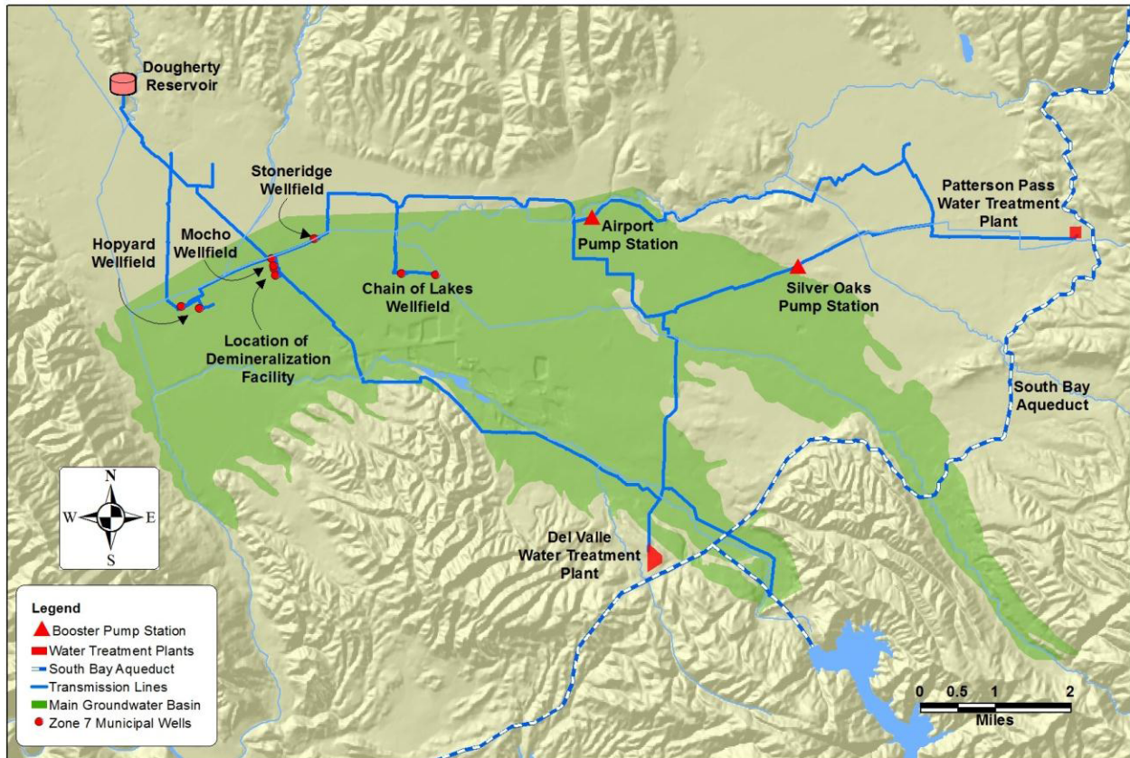
Figure 1-2. Zone 7's Major Treated Water System Facilities
