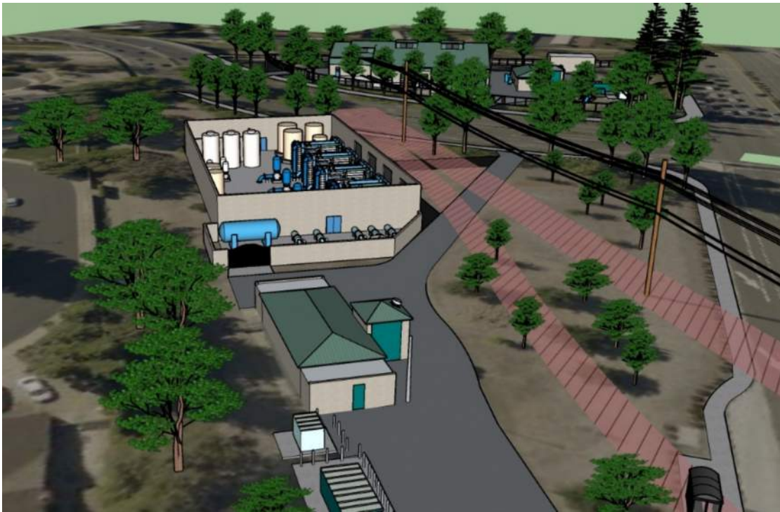
Figure 24 Centralized Mocho Wellfield Treatment at Mocho 3 – RO for Mocho 1, 2, and 3 PFAS
